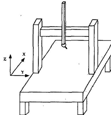
Fig. 1. Schematic diagram of CMM.
