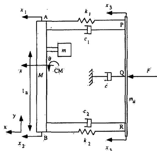
Fig. 2. Two-dimensional model of a CMM with the force  $F$  acting at  $Q$ .
